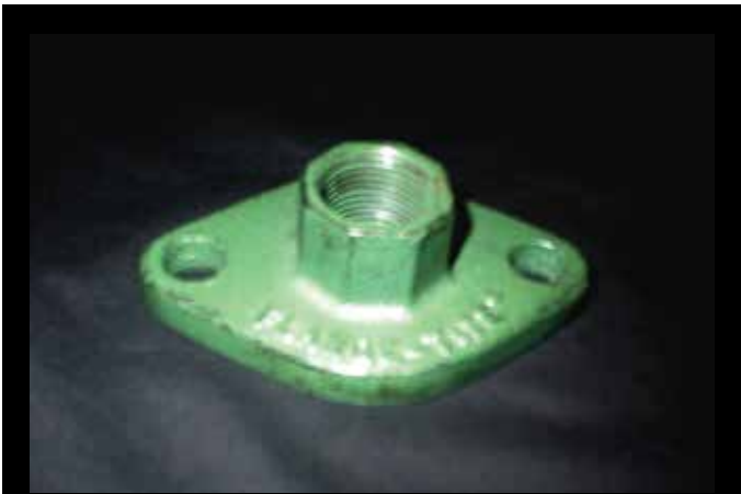
Figure 15: The first of many FLANGE-TITE flange designs. An octagon grip surface and a stronger iron means that no special tools are needed for installation – any adjustable or pipe wrench can easily grip the “wrench boss”.
