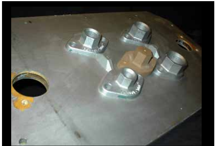
Figure 16: The 1st flange tool pattern sits compared to the 1st flange pattern with 4 different sizes – 3/4” – 1-1/2” female pipe thread.
